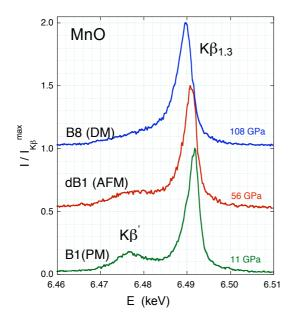
**Figure 1**Mn K-edge x-ray emission spectra of MnO at high pressures showing a significant modification of magnetic moment evident from the changes in K $\beta$ ' as pressure increases. These spectral changes occur abruptly at 30 GPa and 105 GPa suggesting the first-order electronic phase transitions.
