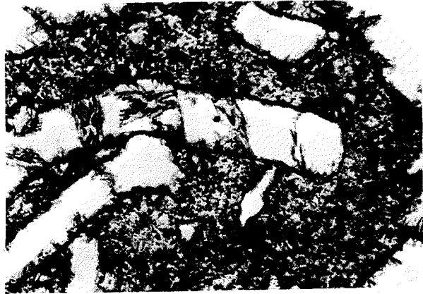
Fig. 1. Inter-particle shear in 71KHCP particle, mixture with Cu (weight content 40 %) ( \times 300 ).
