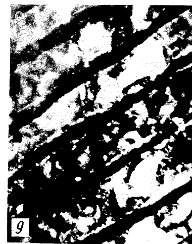
Fig. 2. Electron microphotographs of structures before (a—d) and after (e—g) hydrostatic pressing ( \times 20000 ); a, f—higher bainite structure; b, e—lower bainite structure; c—dark-field image in cementite reflex; d—thin-plate pearlite of mixed structure; g—annealed plate pearlite.
