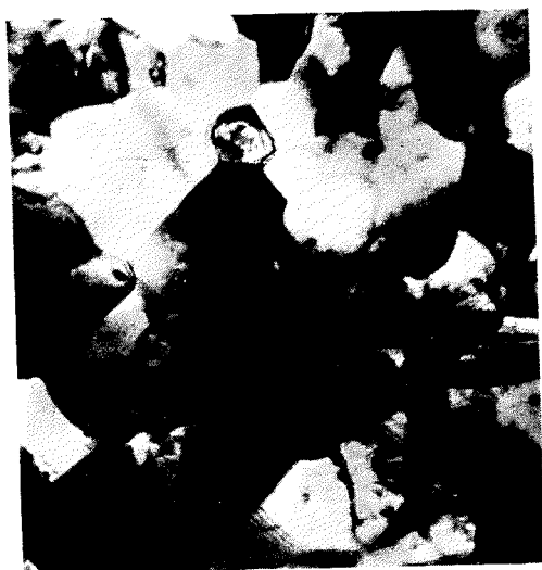
Fig. 1. Structure of 120X3Г3 steel after hydroextrusion, \times 40000 .
