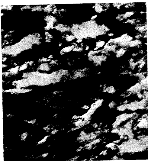
Fig. 1. Structure of 120X3Г3 steel after hydroextrusion, \times 40000 .
