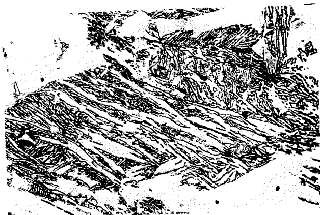
Fig. 3. Martensite crystals with austenite plates of bcc-fcc transformation induced by dynamic pressure of 13 GPa ( \times 500 ).
