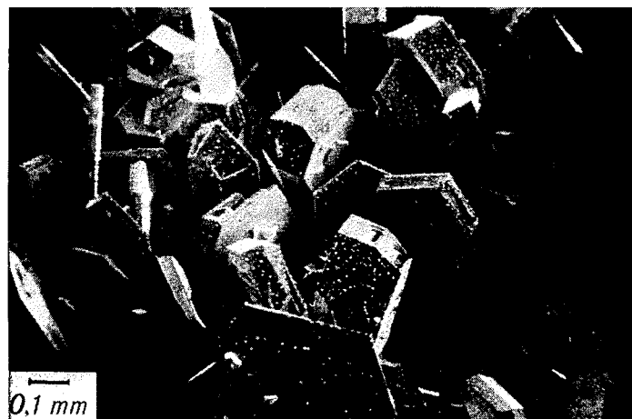
Fig. 4. GaN crust with plate-like crystals on its internal surface — 12 kbar at 1400 °C.
