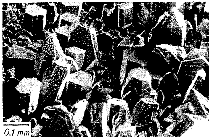
Fig. 6. Intermediate region between plates and columns — 12 kbar and 1300 °C.
