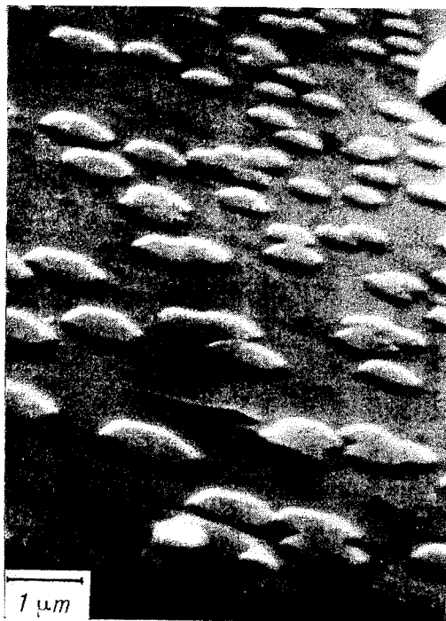
Fig. 9. Two-dimensional nucleation on [0001] face.
